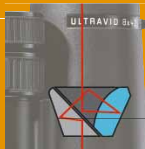
Mirror layer of Leica HighLux-System HLS™
